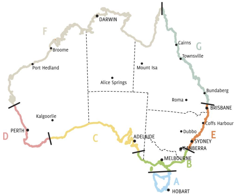
Figure 5.1.1. Marine borer hazard coastal zones. Zone G is the most hazardous.
