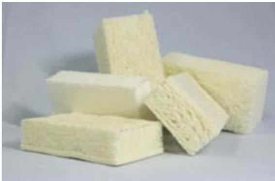
New wood fibre-based insulation materials and sprayable insulation foams will replace products made of non-renewable or poorly recyclable raw materials. These mass producible materials lower energy consumption at the production stage, and reduce the products' carbon footprint.
