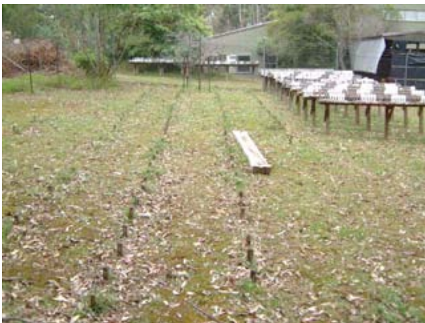
Figure 1. Natural durability test stakes on 23 September 2003 at Pennant Hills
