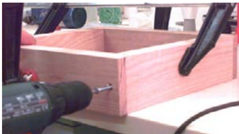
Figure 4.9: Arranged components of a model window frame being clamped (a) and a single screw being driven into the overlapping rebate to fix the butt joint (b).
