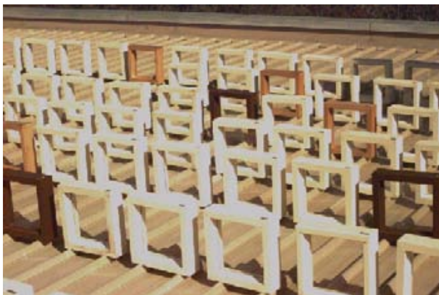
Figure 4.10: Summer exposure of model window frames on the roof of the Clayton laboratory.
