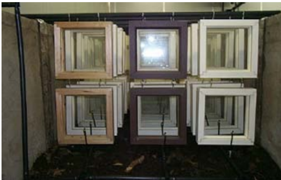
Figure 4.11: Exposure of model window frames during the nine cooler months of the year in the AFS.
