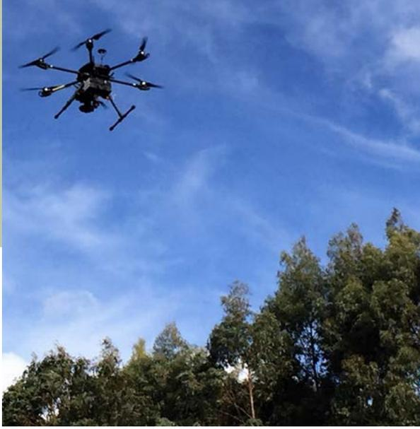
UAV's fitted with specialist cameras and 'koala-identification' algorithms to detect koalas before tree harvesting.
