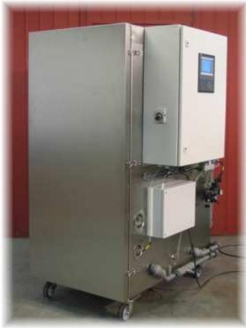
Figure 2.1: Example of a 1m<sup>3</sup> test chamber.
