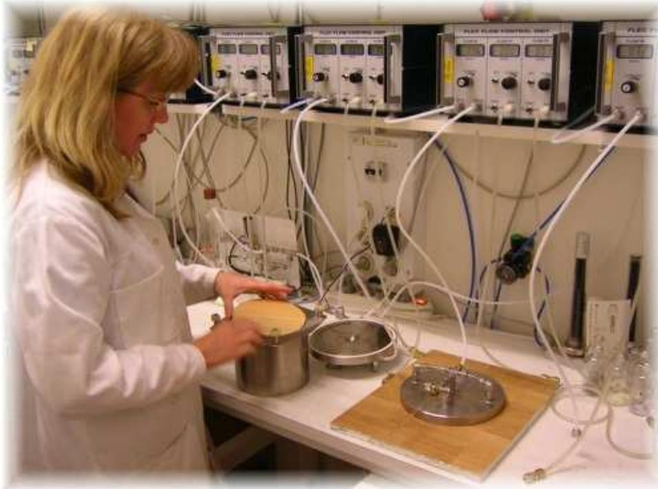
Figure 2.2: FLEC micro-chambers at S.P. Technical Research Institute of Sweden.
